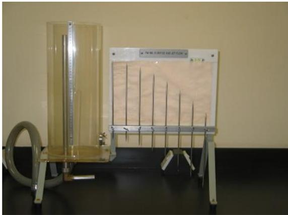
**Device Name:** Orifice and jet flow apparatus
