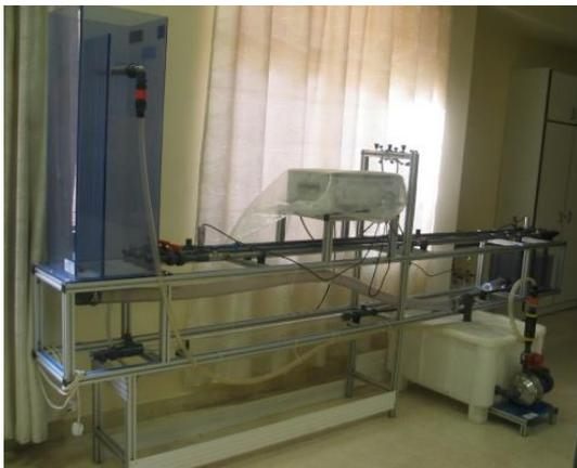
**Device Name:** Computer Controlled Water Hammer Unit, with SCADA
