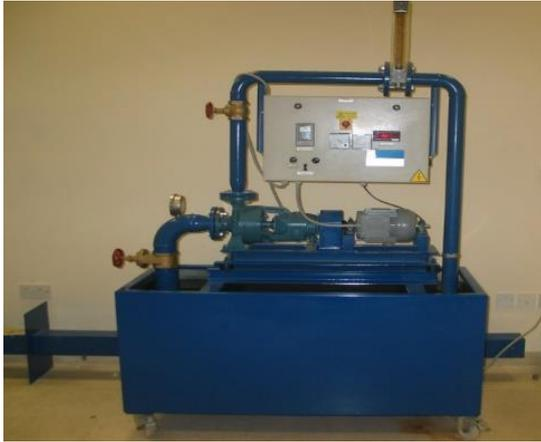
**Device Name:** Centrifugal Pump Test Rig.
