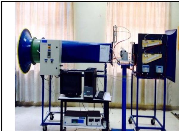
**Device Name:** Open Circuit wind Tunnel.
