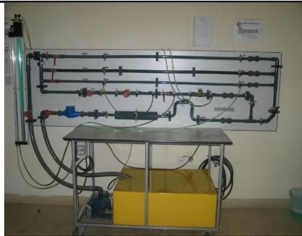
**Device Name:** Piping loss test panel.
