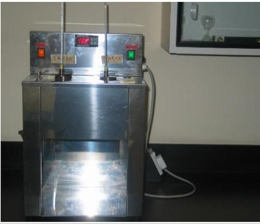
**Device Name:** Two tube Saybolt viscometer
