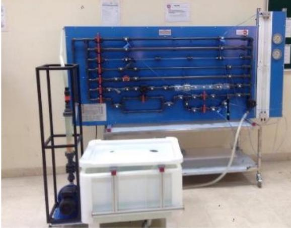
**Device Name:** fluid friction in pipes with basic hydraulic feed system.
