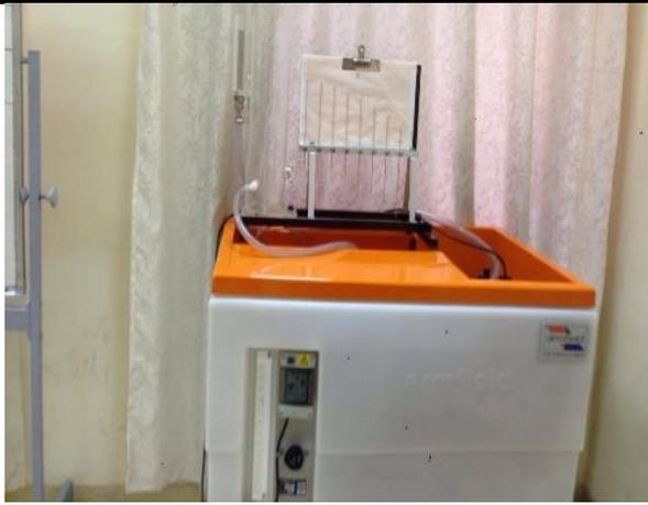
**Device Name:** Orifice and jet flow apparatus
