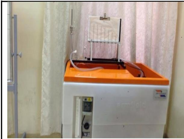
**Device Name:** Orifice and jet flow apparatus
