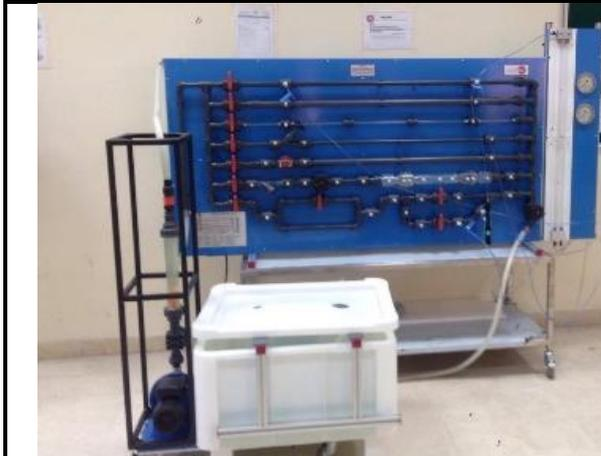
**Device Name:** fluid friction in pipes with basic hydraulic feed system.
