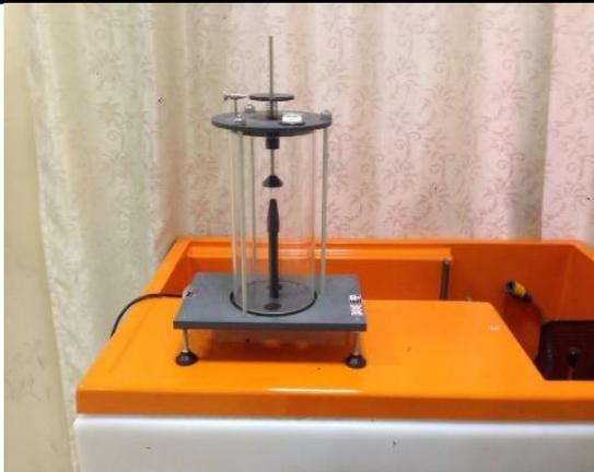
**Device Name:** Impact of water jet apparatus.
