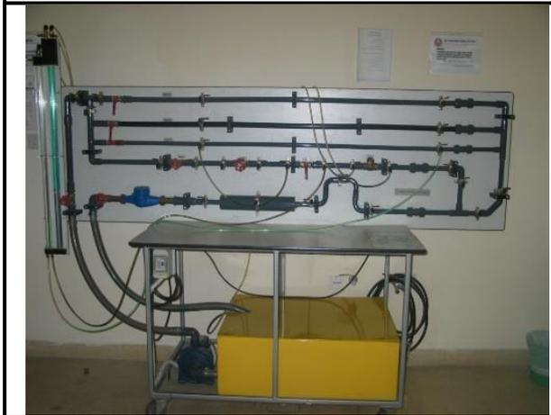
**Device Name:** Piping loss test panel.
