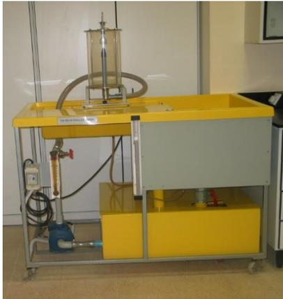
**Device Name:** Impact of water jet apparatus.
